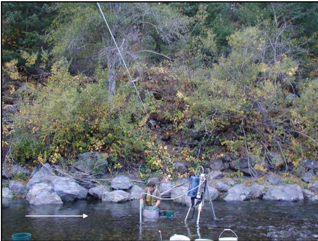
24 inch McNeil sampler and backpack mounted permeability pump on the mainstem at Hyampom Road.
