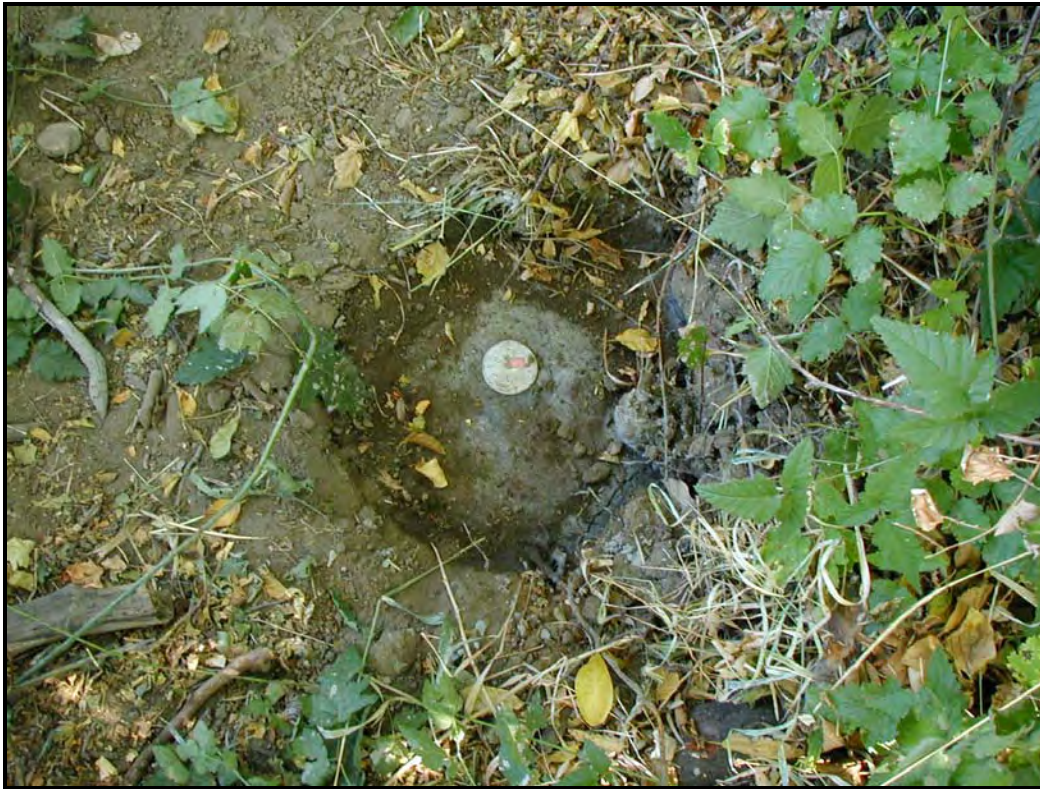
GMA benchmark: aluminum capped 5/8 in. rebar in concrete (HCNH BM #2).
