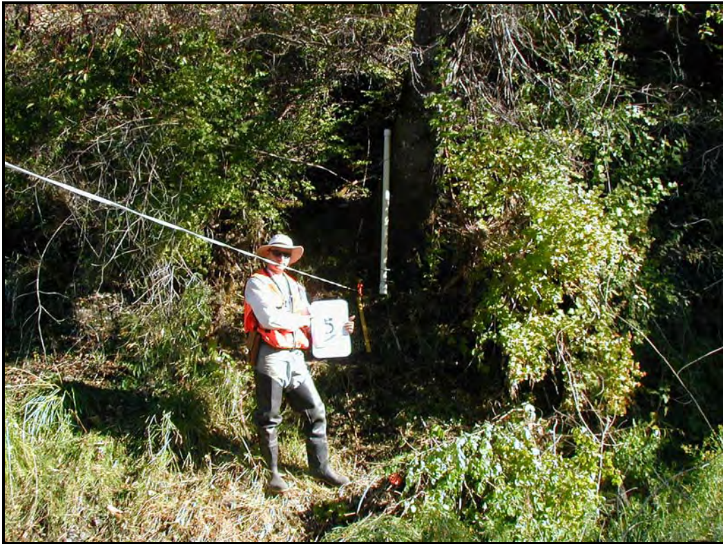
Left bank Cross Section 5 (HCHY), showing slope-area crest gage for recording flood peaks.
