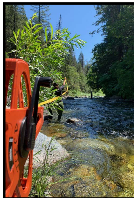
Figure 2. (Right): RCD and WRTC staff work together to extend a measuring tape downstream to calculate gradient on Stuart's Fork during a Stream Condition Inventory (SCI).
