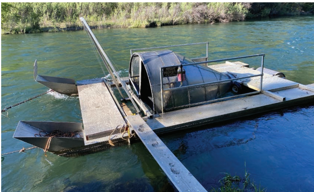
Figure 1. A rotary screw trap fishes the Trinity River downstream of Junction City
